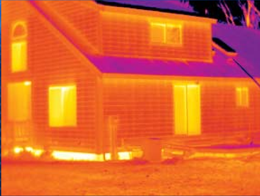
A thermogram of a house
